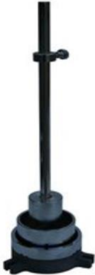
Compaction rammer for compacting 50 mm diameter samples
